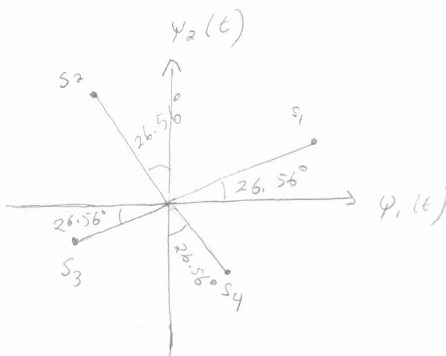
This is QAM, since signal vector lengths of  $s_1 \dots s_4$  are different, additionally spacings between signal vectors seem to be optimum, since
